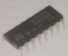
The ULN2003 is an array of seven NPN Darlington transistors capable of 500 mA, 50 V output. It features common-cathode fly back diodes for switching inductive loads. It can come in PDIP, SOIC, SOP or TSSOP packaging. In the same family are ULN2002A, ULN2004A, as well as ULQ2003A and ULQ2004A, designed for different logic input levels.
